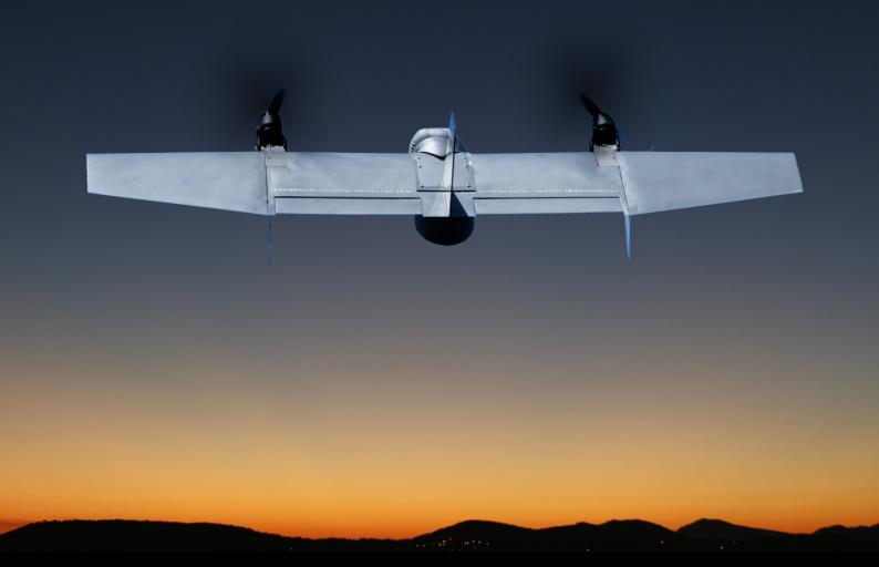
CorvoX is a next generation military grade SUAS, featuring an innovative, thrust vectored VTOL configuration that delivers class leading endurance in extreme weather conditions.
